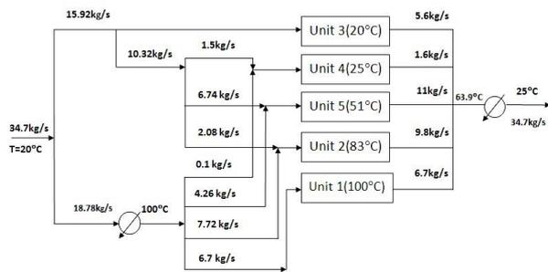
**Figure 6.** Non-isothermal stream mixing for water network of refinery
