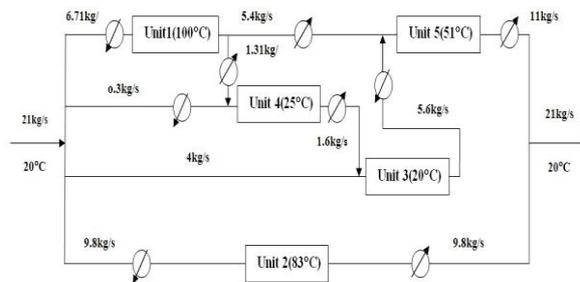
**Figure 8.** Final network with maximum reuse of water
