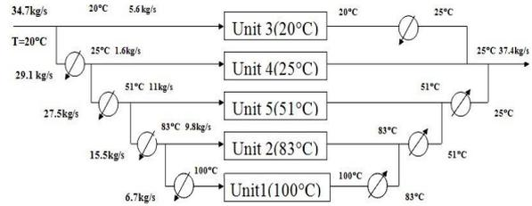
**Figure 3.** Isothermal stream mixing for water network of refinery
