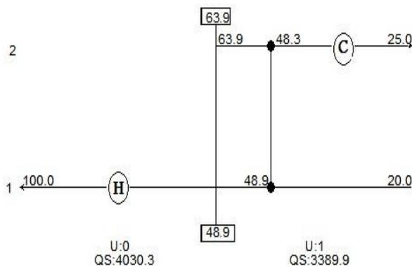
**Figure 7.** Heat exchanger network for non-isothermal stream mixing
