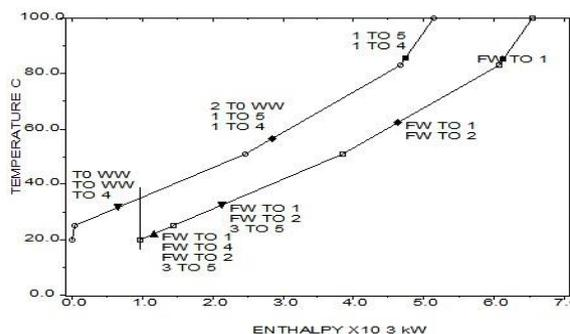
**Figure 9.** Energy composite curve for new water network
