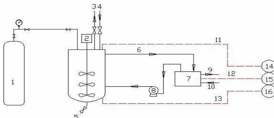
**Figure 1.** Experimental set up: 1-H<sub>2</sub> Cylinder, 2-Stirrer motor, 3-Vent, 4-Feed inlet, 5-Drainage and sampling, 6-Outlet cooled oil, 7-Oil bath, 8-Oil pump, 9-Outlet warmed water, 10-Inlet cooled water, 11-Reactor pressure signal, 12-Oil bath temperature signal, 13-Reactor temperature signal, 14-Reactor pressure recorder, 15-Oil bath temperature recorder, 16-Reactor temperature recorder
