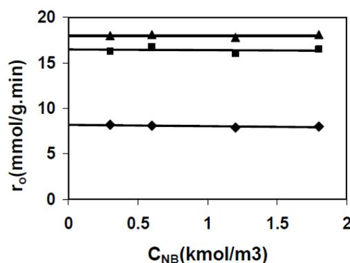
Figure 4. Effect of the concentration of nitrobenzene on initial rate. Reaction conditions: T=323 K, P=5 bar, stirring speed=1500rpm,  $\blacklozenge$ -  $m_{Pd/\gamma-Al_2O_3}=2.5$  g/dm<sup>3</sup>,  $\blacksquare$ -  $m_{nano-Pd}$  on  $\gamma-Al_2O_3=0.8$  g/dm<sup>3</sup>,  $\blacktriangle$ -  $m_{Pd/C}=2.5$  g/dm<sup>3</sup>
