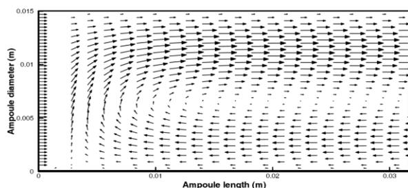
**Figure 4.** Flow patterns for flow transition from pure diffusion/advection to full circulatory convection ( $P=0.03$  atm, others are the same as in Figure 3).
