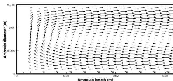
**Figure 5.** Flow patterns for full circulatory convection near the two ends. ( $P=0.1$  atm, others are the same as in Figure 3).
