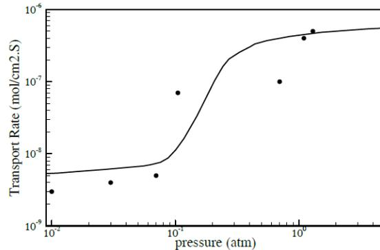
**Figure 2.** Transport rate as a function of total pressure, Discrete points are the experimental data, Ref. [4].
