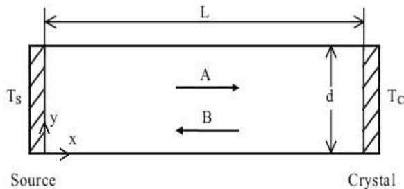
**Figure 1.** Schematic and coordinates of closed ampoule
