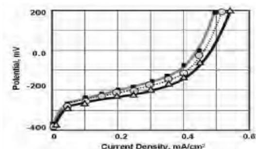
**Figure 4.** Polarization curves of three TP/MWNTs/PEI, GOx, Nafion electrodes. 20 mM phosphate buffer, pH 6.9, 0.1M KCl, 20 mM glucose 20 C. 0.1 cm<sup>2</sup> electrodes.
