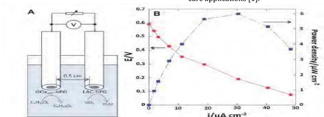
**Figure1.** Scheme of the enzymatic biofuel cell set up. B: Polarisation and power density curve of the GOx<sub>ads</sub> hPG and LAC-hPG biofuel cell. The power and the current density refer to the total superficial surface area of the electrodes used (0.03 cm<sup>2</sup>).
