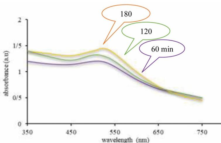
**Figure 1:** UV-Vis absorption spectrum of CuNPs biosynthesis at different time intervals.
