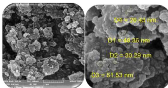
**Fig 2:** SEM image of the biosynthesized CuNPs by using pistachio hull extract.
