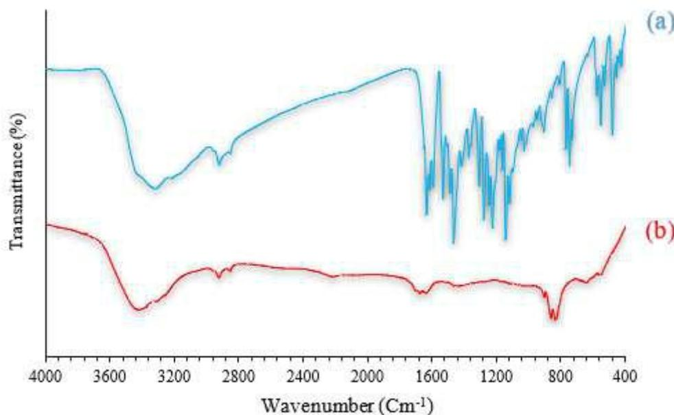
Fig 3: FT-IR of SL (a) and SSC (b).
