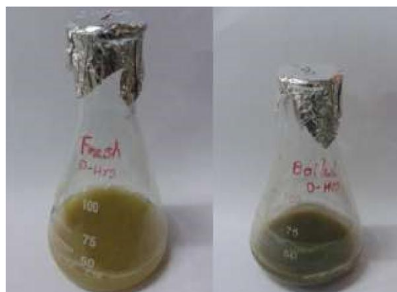
Figure 1. The colour changes observed on synthesis of silver nanoparticles on 0 hrs incubation of fresh and boiled stem extracts of Caralluma fimbriata
