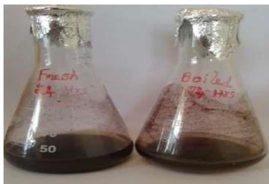
Figure 3. The colour changes observed on synthesis of silver nanoparticles on 24 hrs incubation of fresh and boiled stem extracts of Caralluma fimbriyata
