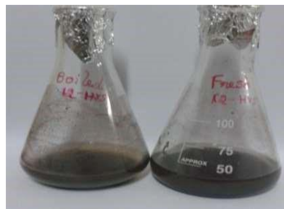
Figure 2. The colour changes observed on synthesis of silver nanoparticles on 12 hrs incubation of fresh and boiled stem extracts of Caralluma fimbriata
