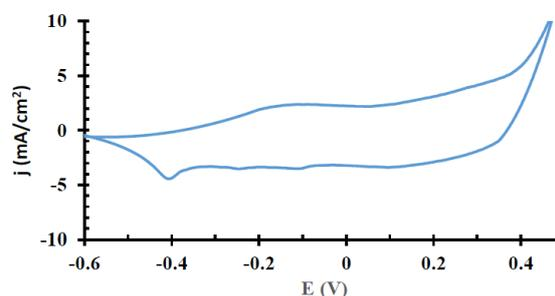
**Figure 1.** Catalyst cyclic voltammogram of Pd-Co/Gr into a KOH solution 1 M with scanning speed equal to 50 mV.s<sup>-1</sup>
