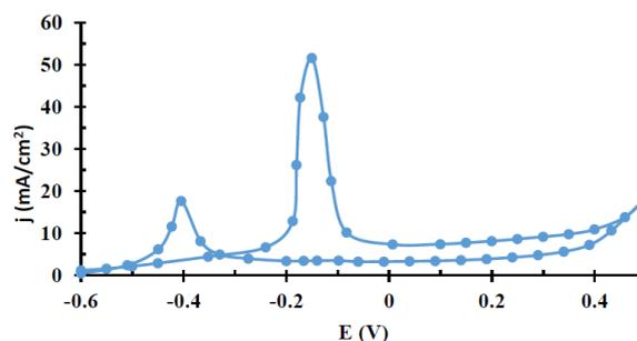
**Figure 2.** Catalyst cyclic voltammogram of Pd-Co/Gr into a KOH 1 M and ethanol 2 M solutions with scanning speed equal to 50 mV.s<sup>-1</sup>
