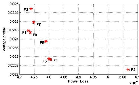
**Figure 7.** Pareto front NSGA-II Algorithm, Voltage Profile- losses.
