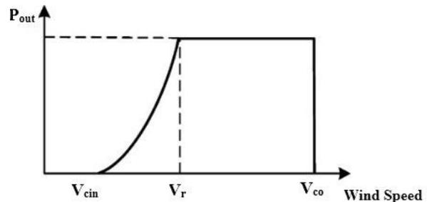
Figure 1. Wind turbine power curve.
