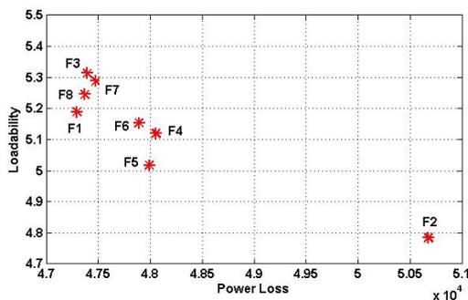
**Figure 8.** Pareto front NSGA-II Algorithm, Loadability- losses.
