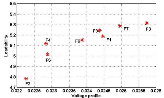
**Figure 9.** Pareto front NSGA-II Algorithm, Loadability- Voltage Profile.
