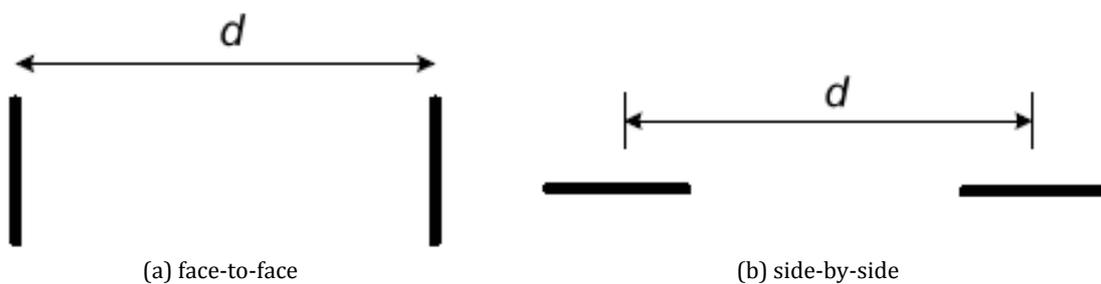
**Figure 5.** Antenna orientations for time domain measurements.
